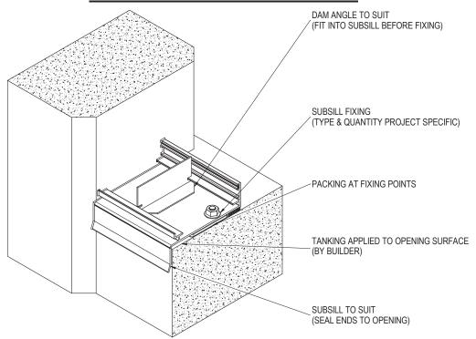
1. INSTALL SUBSILL INTO OPENING WITH DAM ANGLE FITTED. PACK SUBSILL LEVEL THEN FIX TO STRUCTURE. SEAL SUBSILL ENDS TO STRUCTURE.
