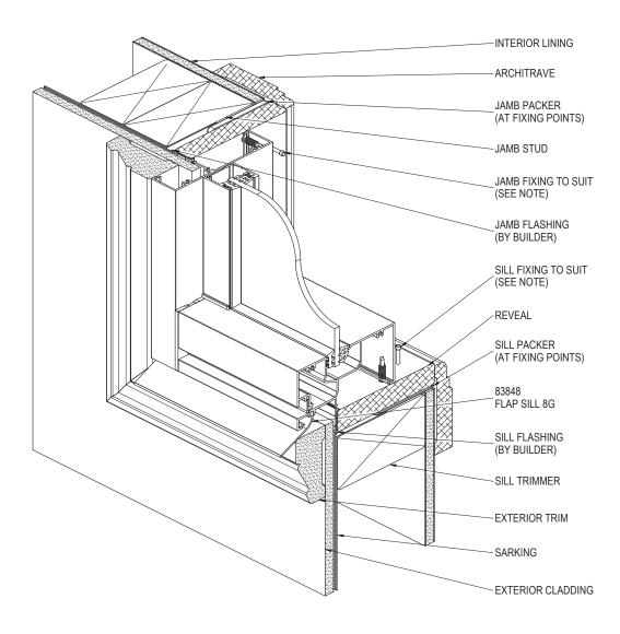
NOTE: FOR SITE CLASSIFICATIONS OF UP TO AND INCLUDING 'N6' OR SIMILAR, FIXINGS ARE TO BE AT 450mm CENTRE MAXIMUM, FOR SITUATIONS IN EXCESS OF THIS THE FIXINGS ARE TO BE AT 300mm CENTRES MAXIMUM. FIXING SIZE TO BE EQUIVALENT TO A  $\oslash$  2.2mm STEEL NAIL MIMIMUM.
