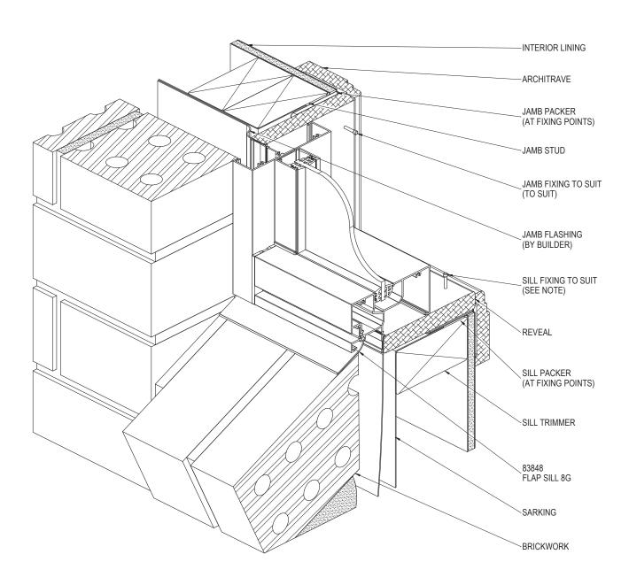
NOTE: FOR SITE CLASSIFICATIONS OF UP TO AND INCLUDING 'N6' OR SIMILAR, FIXINGS ARE TO BE AT 450mm CENTRE MAXIMUM, FOR SITUATIONS IN EXCESS OF THIS THE FIXINGS ARE TO BE AT 300mm CENTRES MAXIMUM. FIXING SIZE TO BE EQUIVALENT TO A  $\emptyset$ 2.2mm STEEL NAIL MIMIMUM.
