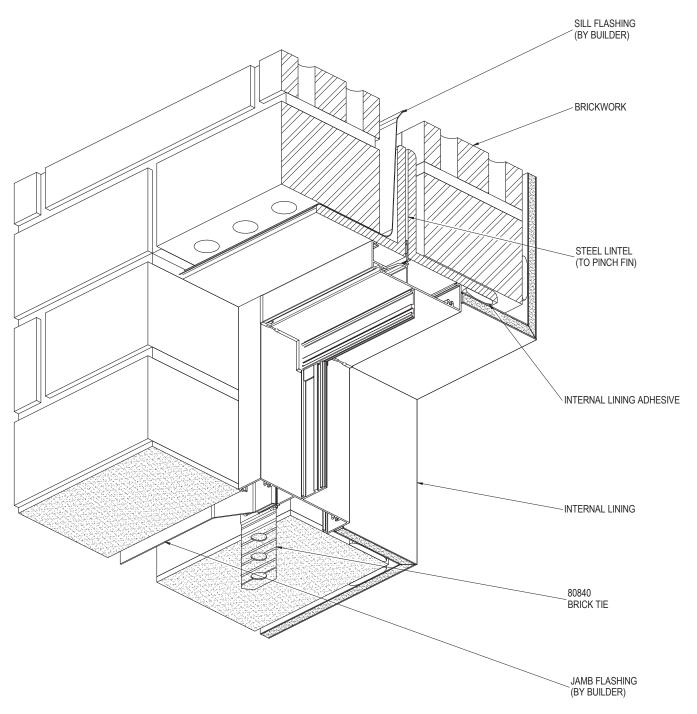
NOTE: FOR SITE CLASSIFICATIONS OF UP TO AND INCLUDING 'N6' OR SIMILAR, FIXINGS ARE TO BE AT 450mm CENTRE MAXIMUM, FOR SITUATIONS IN EXCESS OF THIS THE FIXINGS ARE TO BE AT 300mm CENTRES MAXIMUM. FIXING SIZE TO BE EQUIVALENT TO A  $\emptyset$ 2.2mm STEEL NAIL MINIMUM.
