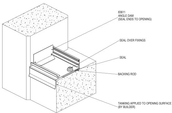
2. APPLY SEALANT TO VERTICAL FACE OF DAM ANGLE AND ALSO TO THE FLOOR OF THE SUBSILL. POSITION DAM ANGLE AGAINST THE STRUCTURE. SEAL ALL JOINTS BETWEEN THE ANGLE AND SUBSILL. SEAL ALL JOINTS BETWEEN ANGLE AND SUBSILL. SEAL OVER FIXINGS AND UNDER SUB SILL TO STRUCTURE.
