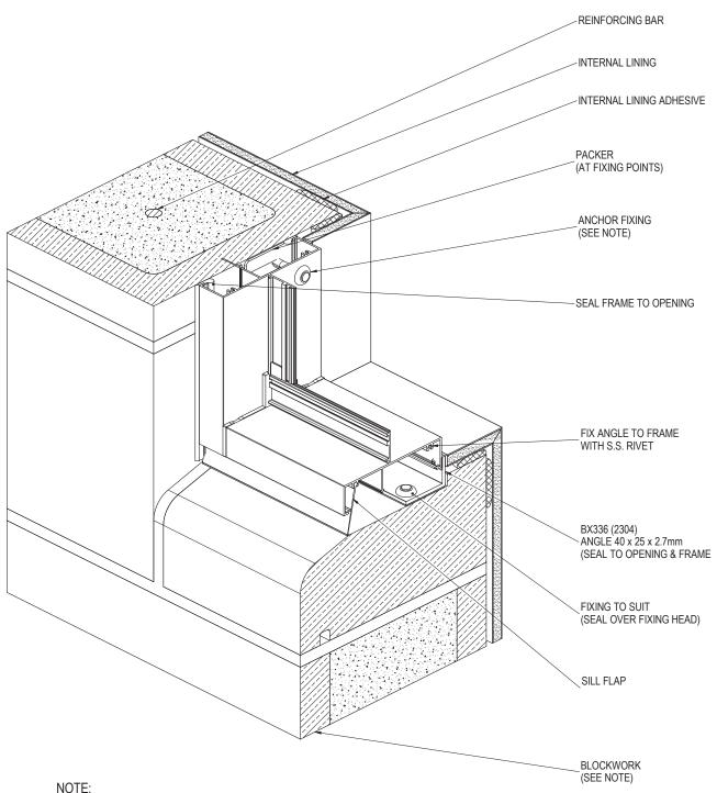
SURFACE OF BLOCKS TO WINDOW OPENING MUST BE TANKED WITH A SUITABLE SEALER TO PREVENT INGRESS OF MOISTURE. ENSURE SURFACES TO BE SEALED ARE SOUND, CLEAN, DRY AND FREE FROM ANY CONTAMINANTS BEFORE SEALING.
