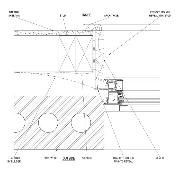
FIXINGS: UP TO AND INCLUDING SITE CLASSIFICATION OF N6, C4 (3.0 kPa) FIXINGS ARE TO BE AT 450mm CENTRE MAXIMUM. FOR SITUATIONS IN EXCESS OF THIS THE FIXINGS ARE TO BE AT 300mm CENTRES MAXIMUM. FIXING SIZE TO BE EQUIVALENT TO A Ø2.2mm STEEL NAIL MINIMUM.
