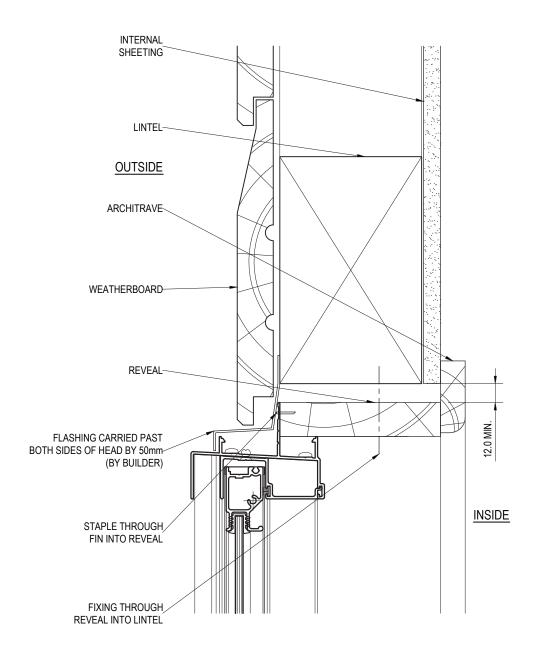
FIXINGS: UP TO AND INCLUDING SITE CLASSIFICATION OF N6, C4 (3.0 kPa) FIXINGS ARE TO BE AT 450mm CENTRE MAXIMUM. FOR SITUATIONS IN EXCESS OF THIS THE FIXINGS ARE TO BE AT 300mm CENTRES MAXIMUM. FIXING SIZE TO BE EQUIVALENT TO A Ø2.2mm STEEL NAIL MINIMUM.
