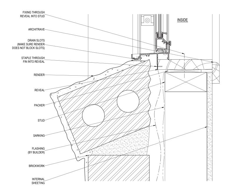
FIXINGS: UP TO AND INCLUDING SITE CLASSIFICATION OF N6, C4 (3.0 kPa) FIXINGS ARE TO BE AT 450mm CENTRE MAXIMUM. FOR SITUATIONS IN EXCESS OF THIS THE FIXINGS ARE TO BE AT 300mm CENTRES MAXIMUM. FIXING SIZE TO BE EQUIVALENT TO A Ø2.2mm STEEL NAIL MINIMUM.
